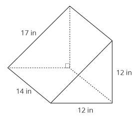
In general, we can find the volume of any prism by multiplying the area of its base times its height. For this prism, the area of the triangular base is  $72 \text{ in}^2$ , so the volume is  $72 \cdot 14$ , or  $1,008 \text{ in}^3$ .
